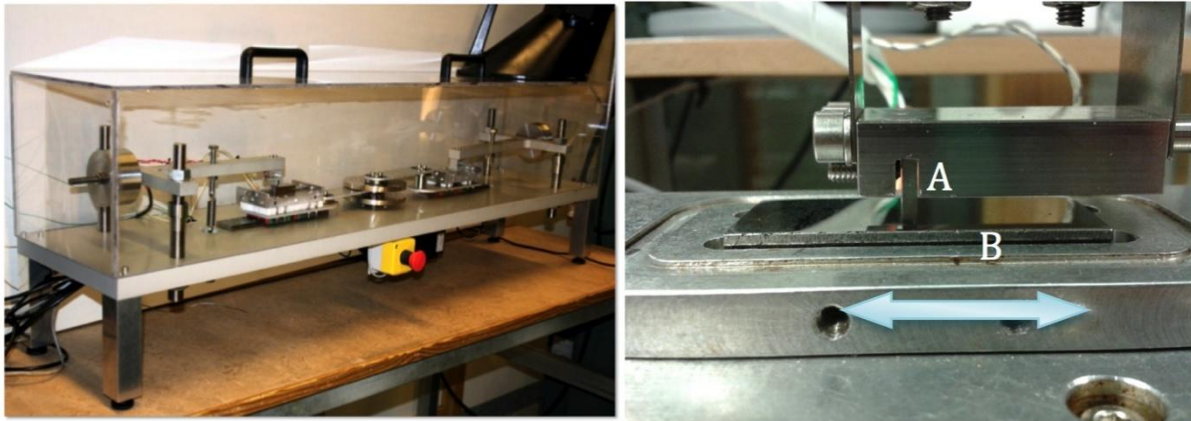
The Helios lab scale test rig, allowing two simultaneous reciprocating sliding tests (left) and a close up of one of the two the sample fixtures (right). Letter A) corresponds to the stationary ring and B) to the reciprocating cylinder sample. The arrow shows the movement of sample B.
