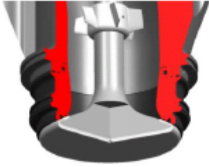
2-stroke exhaust valve
