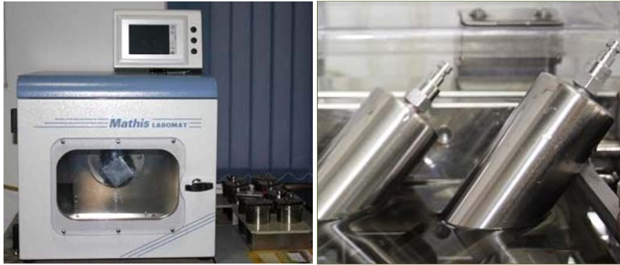
Fig. 6. Enzymatic delignification (of whole lignocellulose) and bleaching (of paper pulp) experiments: General view of the multireactor equipment (left) and detail of the pressurized individual reactors outside the equipment (right).
