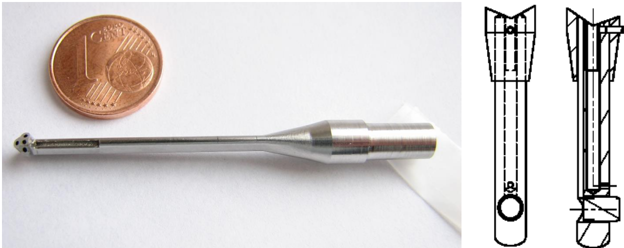
Figure 11: Picture of DLR 5-hole-probe (left) and drawings of VKI FRAP Kulite probe heads (right)
