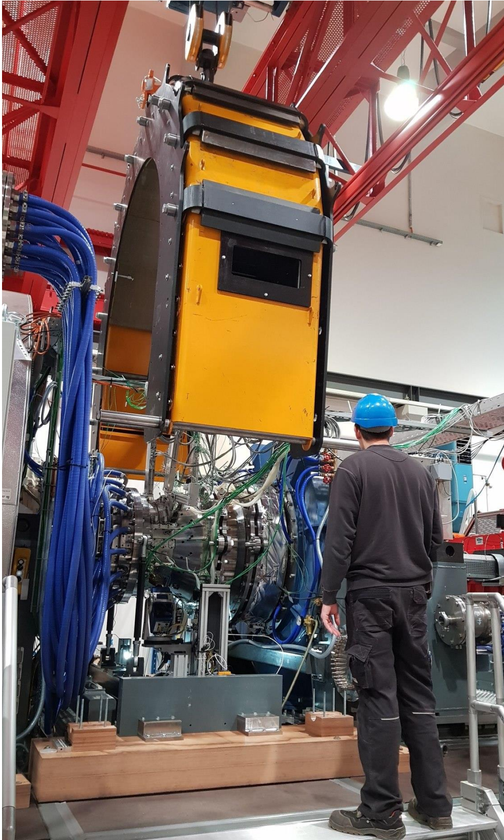
Figure 23: FACTOR rig integration - mounting the containment around the closed & instrumented rig
