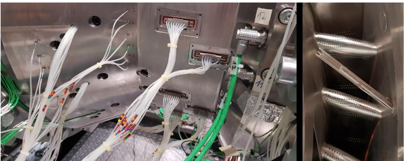
Figure 20: FACTOR rig integration - main casing instrumentation with tubes, connectors and sensors
