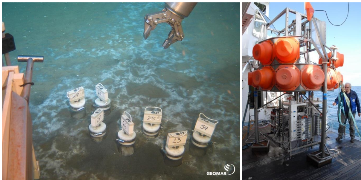
Figure 21: ROV Kiel 6000 is deployed at the seabed to take sediment samples from a bacterial mat patch located within the Hugin Fracture (left). Pore fluids are extracted from the retrieved sediments to determine the chemical composition and origin of formations fluids and dissolved gases seeping through the seabed. Subsequently, a benthic chamber lander is placed at the seabed (right) to measure formation water fluxes and determine emission rates (images provided by P. Linke, GEOMAR).
