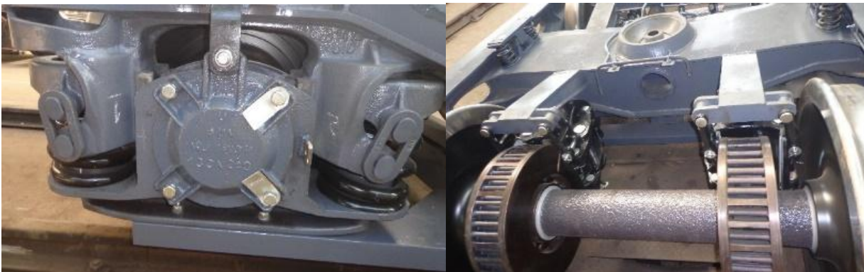
Figure 12: Lateral view showing the double Lenoir links
