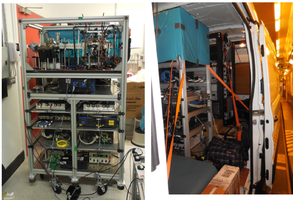
Figure 4.3 The Sr 2 nd generation system in the lab (left, without electronics rack and clock laser subsystem) and on the Eurotunnel train on its way from UBham to PTB (right).
