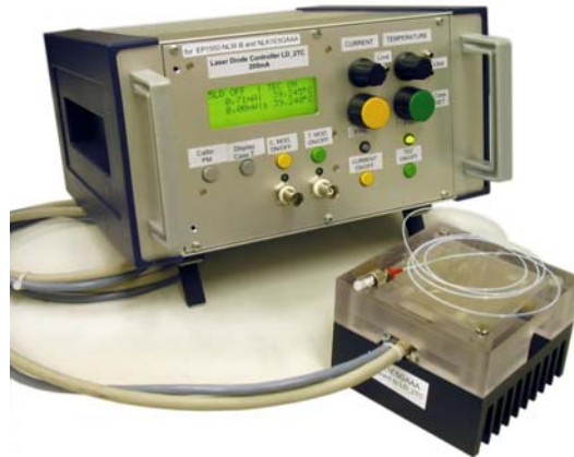
Figure 1.2 The 1389 nm repumper laser for the Yb clock
