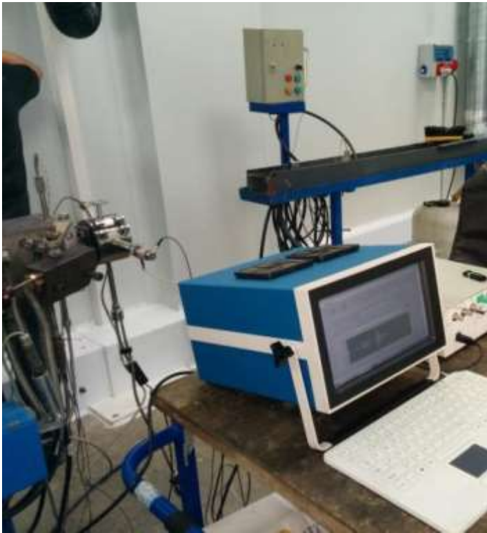
Figure 3.1.6.1: Global view of the ultrasonic measurement system
