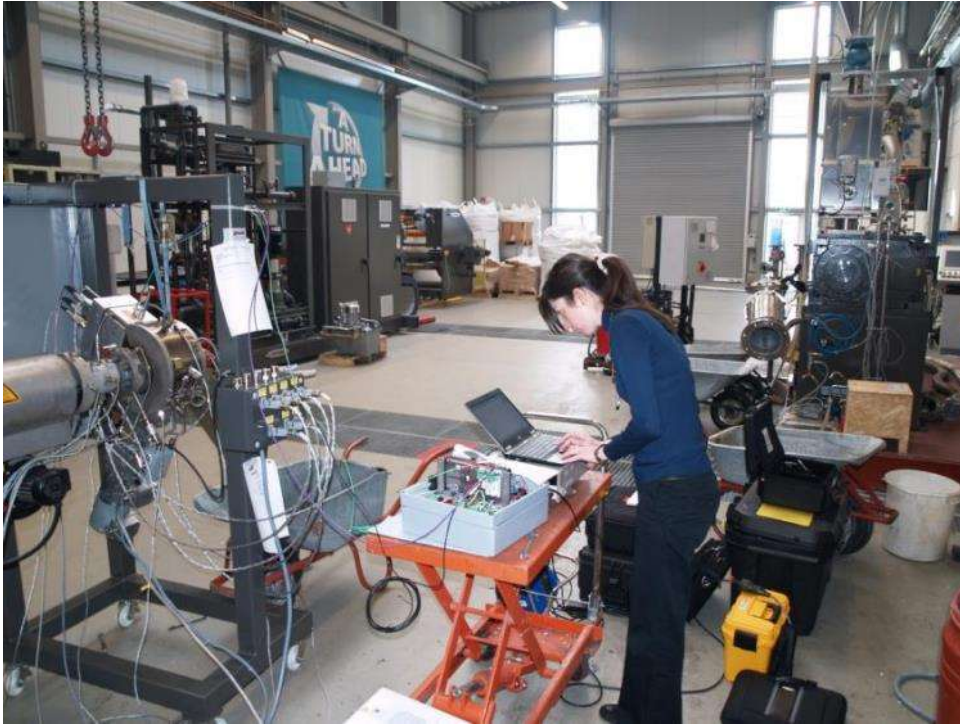
Figure 3.1.3.3: Measurements at Gneuss on a real ONBOX in March 2012 on prototype sensors and measurement and control unit. The measurement and control in this phase are still autonomous.
