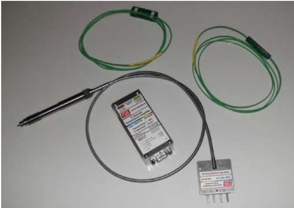
Figure 3.1.2.8: FOS multi point gradient thermometer measuring setup.
