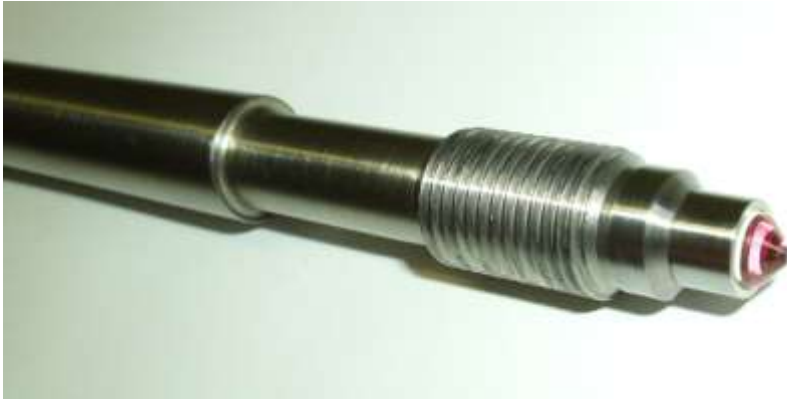
Figure 3.1.5.14: Frontend of FOS ATR-NIR-FO-Probe with sapphire crystal tip.
