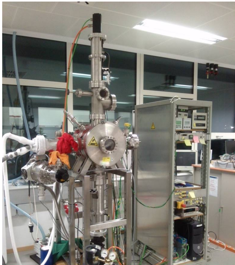
Figure 4-2: AAC SALOTTE: test rig for harmonic gears under thermal vacuum (running at low temperature, seen by iced feed lines for the liquid nitrogen)
