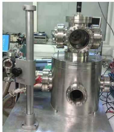
Figure 10. The breadboard vacuum chamber. Bottom chamber is 400mm diameter, top chamber is 200 mm diameter.
