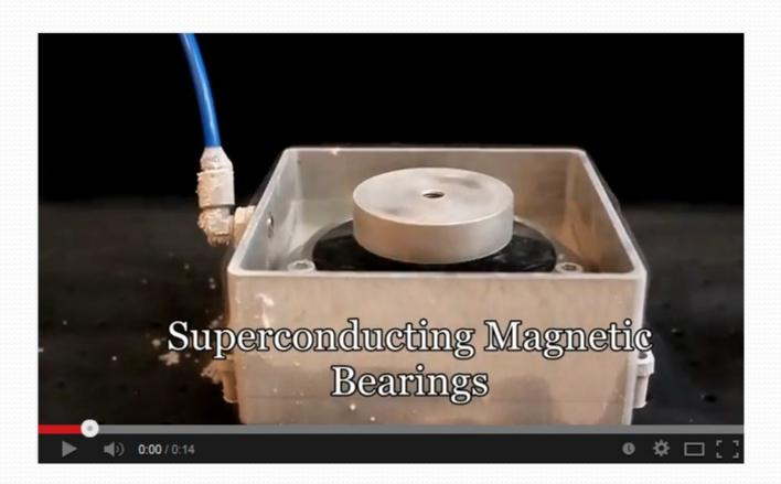
Thrust bearing. Magnet spinning&floating over a superconductor base.
