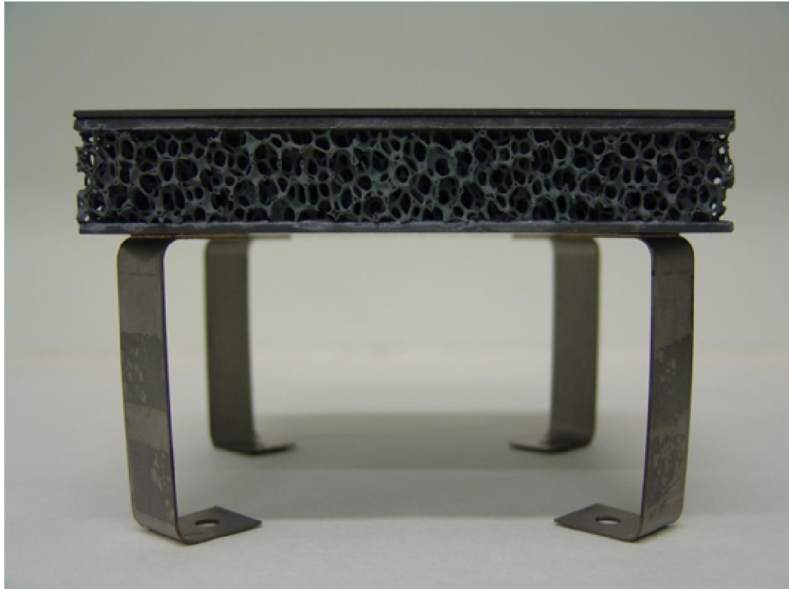
Fig.5.4. The technology sample 150 \times 150 \text{ mm}^2 for load case 2 after the brazing process of the Ti stand offs.
