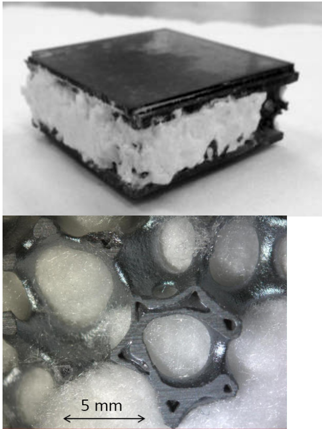
Figure 2.13 On the left a 50x50 [mm] sandwich tile produced filling reticulated SiSiC with oxide fibres. On the right a close view of the foam showing the complete filling of the macroporosity.
