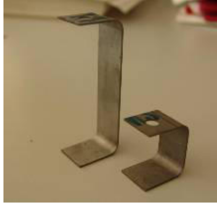
Fig. 5.1. The Ti stand off for load case 1 and 2.
