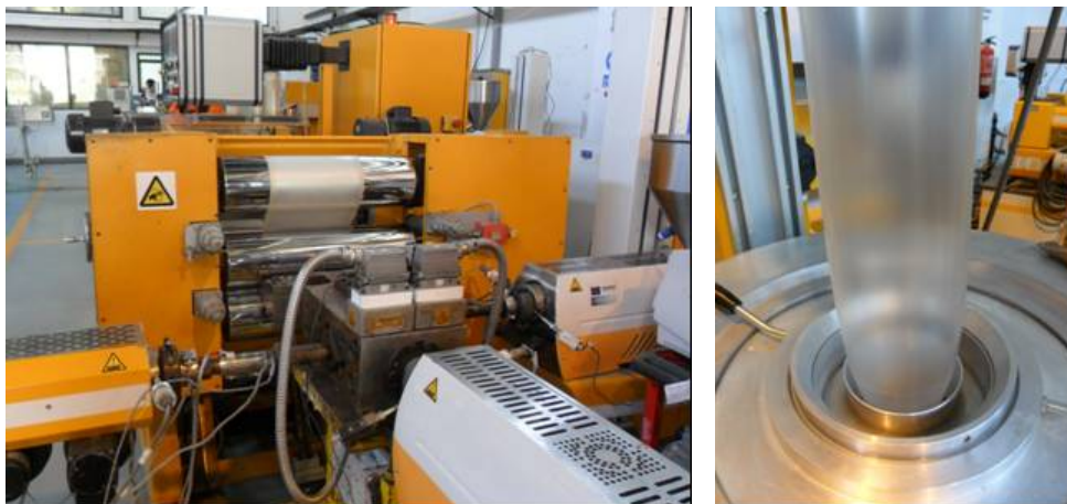
Figure 2-3 . Cast sheet and blown film extrusion of materials developed in the project.
