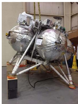
Figure 23 : Morpheus lander with three different laser devices on the top (white) including one flash imaging LiDAR.
