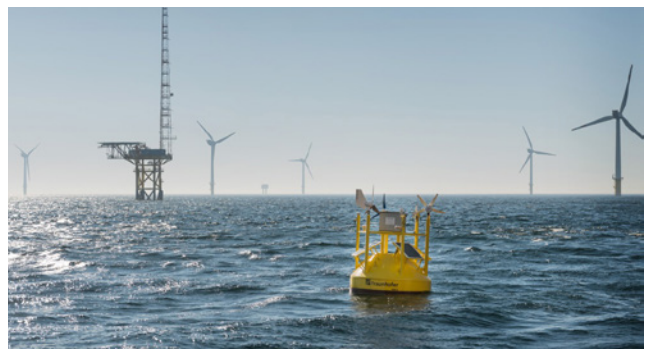
Offshore test of Fraunhofer IWES Wind Lidar Buoy next to FINO1 met. mast 45 km offshore, North Sea.
