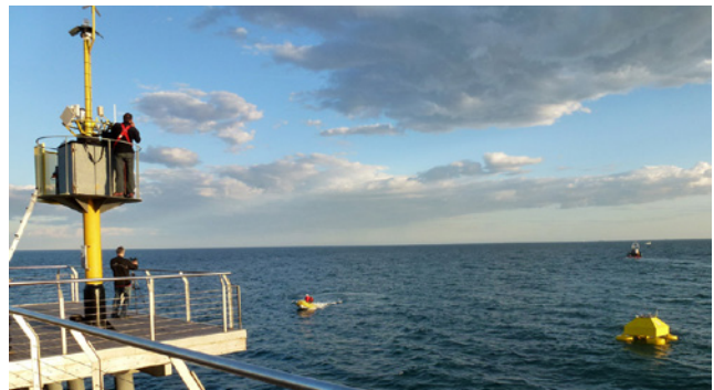
Parallel measurements of the floating lidar and a fixed lidar installed on the Pont de Petroli, Badalona, Catalonia, Spain
