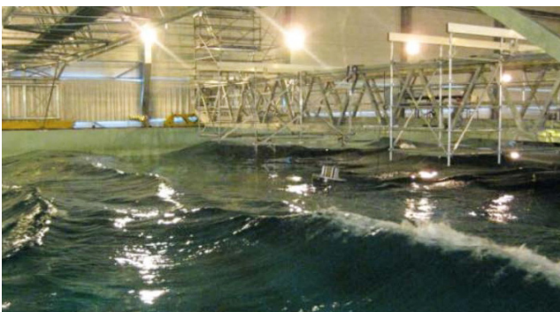
The Tfl elastomer tether mooring system was tested on the Wavebob scale device in the hydrodynamic and ocean engineering tank at ECN.
