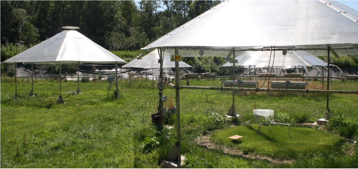
Figure 6. Set-up to test a new infrared heater control based on the energy balance (Antwerp, Belgium)
