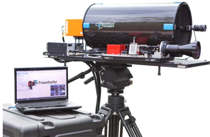
Figure 19. The backscattering spectroscopy system developed within the EMPHASIS project.
