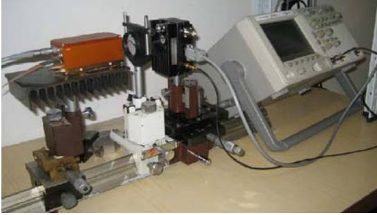
Figure 12. Time response measurement sets with quantum cascade laser (a) and optical parametric oscillator (b).
