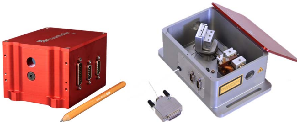
Figure 18. Left: closed EC-QCL module Right: view into interior of EC-QCL module showing the optical grating that is used as wavelength selective element and is mounted on a rotation stage.
