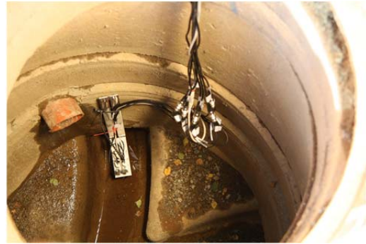
Figure 36. EMPHASIS sewer sensor; Concept and deployment in sewer.
