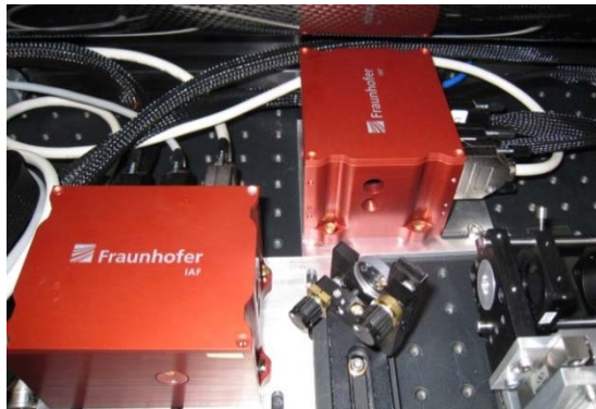
Figure 20. Wavelength range extension by addition of a second laser illumination source covering the range between 1000\text{ cm}^{-1} and 1100\text{ cm}^{-1} . The two beams were overlaid using a dichroitic mirror at 1100\text{ cm}^{-1}
