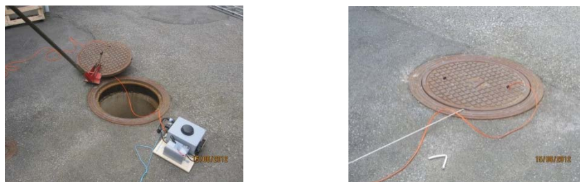
Figure 28. Field-trial with GSM based equipment
