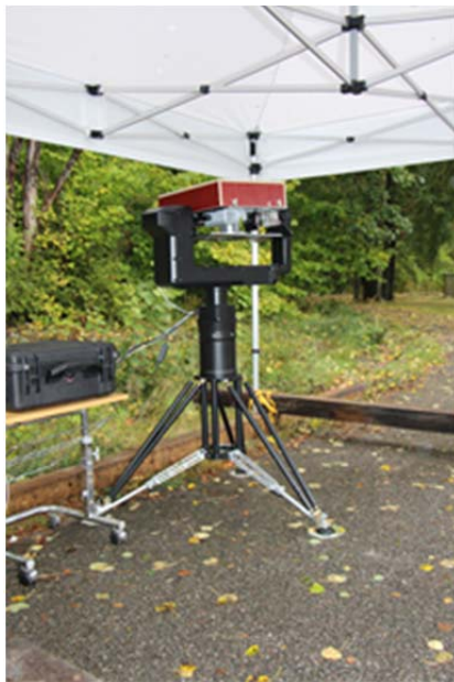
Figure 35. An open path system deployed during the EMPHASIS demonstration for IR detection.
