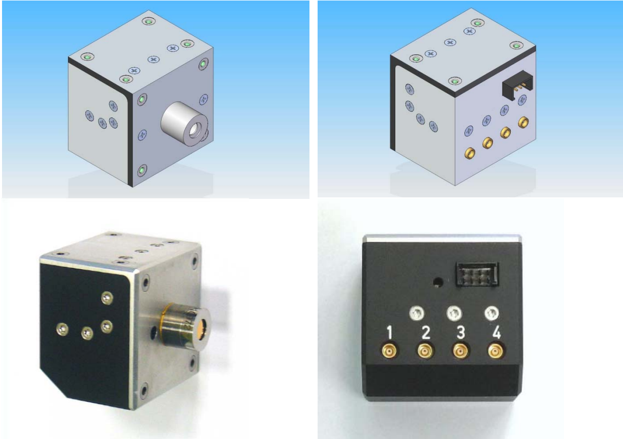
Figure 9. Front and rear view of Emphasis detection module design and its final version.
