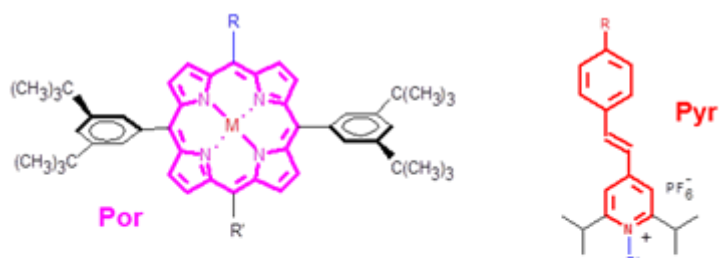
Fig. WP2-2; General formulae for Por-Bb's and Pyr-Bb's included in the project. The substituents R and R' can be varied practically at will. The chromophoric system responsible for the photophysical properties is shown with coloured bold bonds. M can be either 2H or various metals such as Zn, Cu, Ni, Mg, Cd, etc. The blue substituents serve to incorporate the Bb's into the peptide chain.
