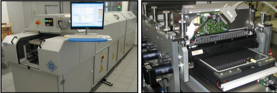
Fig. WP1-1; Views on the 2 nd generation peptide laser printer with 4 from 24 printing units being visible.
