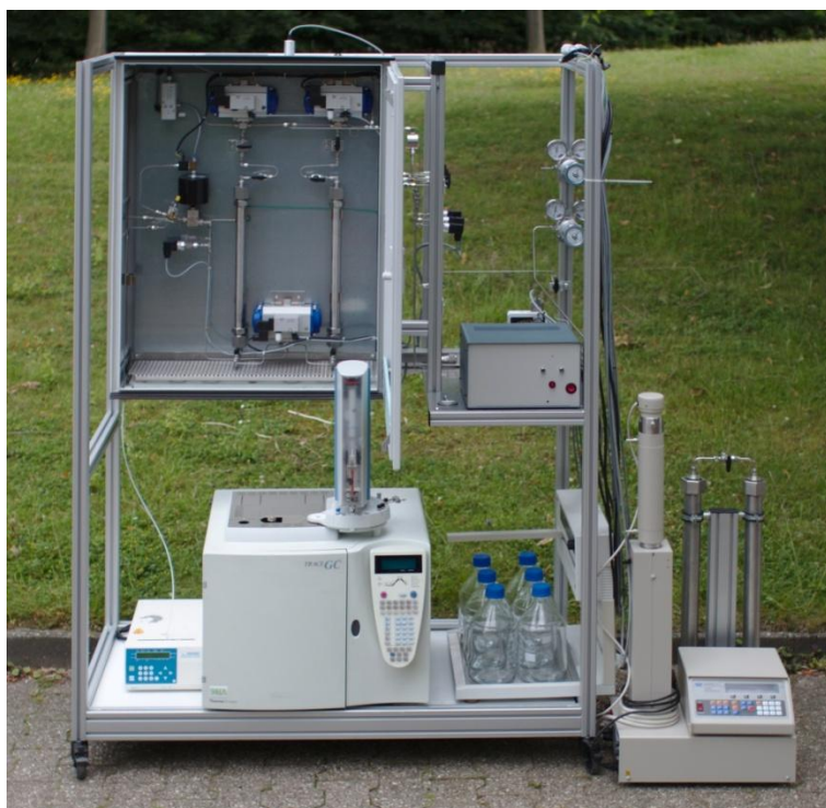
Figure 3: Demonstrator unit for the asymmetric hydrogenation (RWTH)
