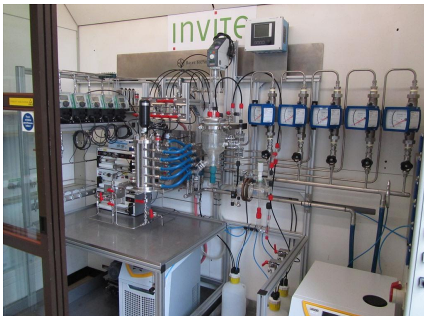
Figure 2: Demonstrator unit for the Buchwald-Hartwig case study at INVITE
