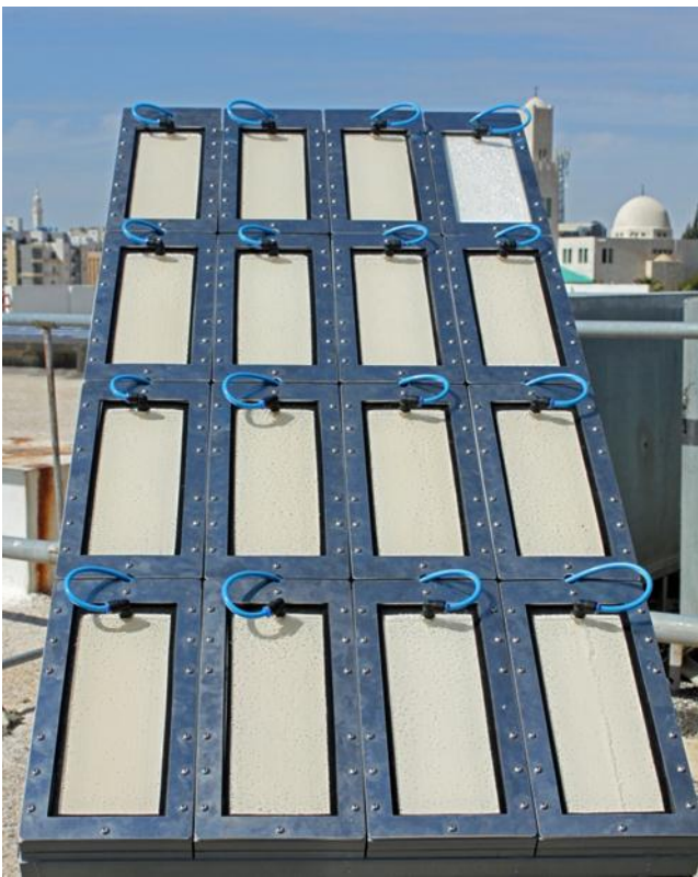
Pilot plant with NATIOMEM membranes in Amman, Jordan
