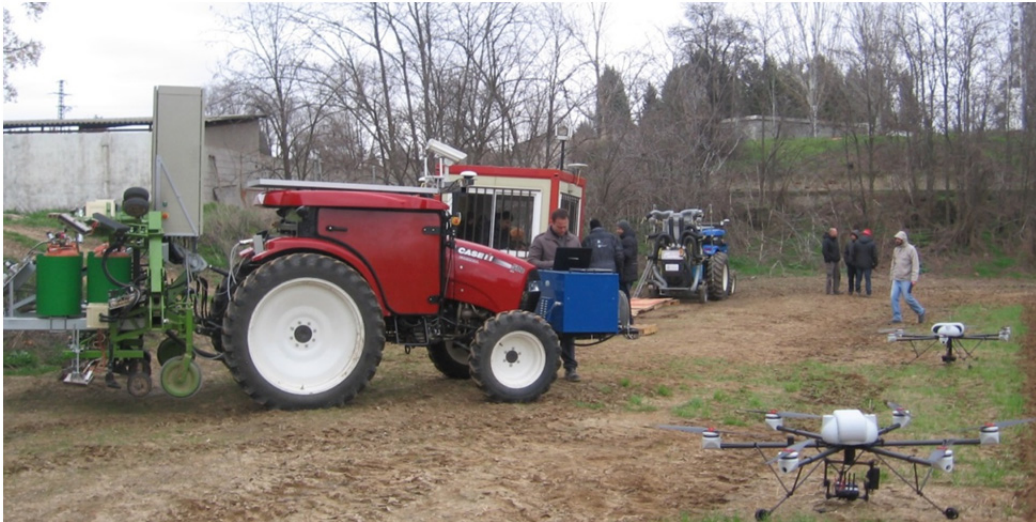
Fig. 1.1. The RHEA fleet: Base station, two GMUs out of three and the two AMUs
