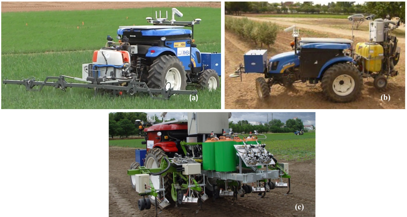
Fig. 4.1: (a) Patch sprayer; (b) Canopy sprayer and (c) Mechanical and thermal device
