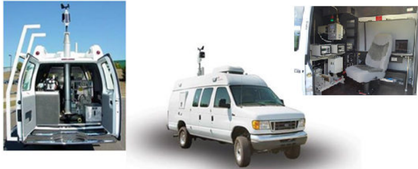
Figure 4: CANBERRA mobile vehicle for in-situ and real-time radiation monitoring.
