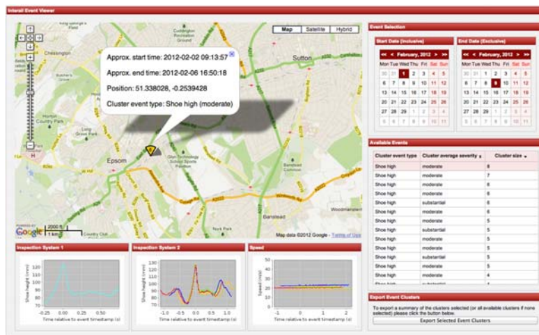
Figure 32 - Web interface to the INTERAIL integrated inspection data (data shown is laser data from South East of England as INTERAIL demonstrations are yet to take place at time of writing).
