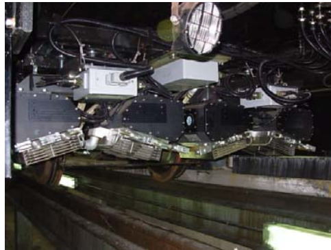
Figure 22 - Rail Profile : triangulation concept layout and real installation
