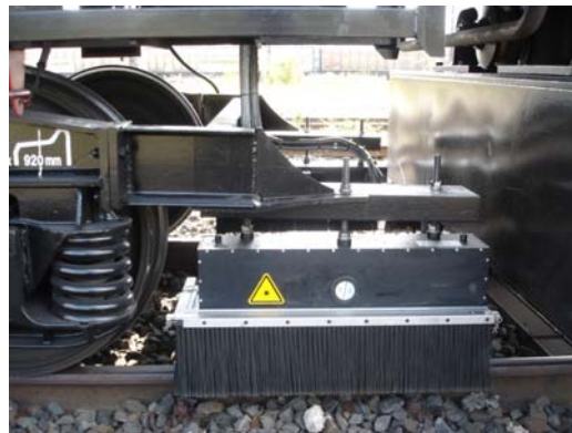
Figure 23 - Rail Corrugation : triangulation concept layout and real installation
