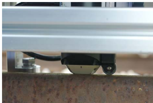
Figure 36 - ACFM probe on top of rail
