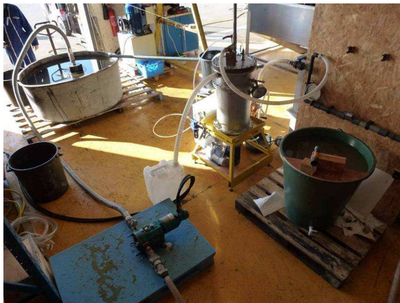
Figure 6: Experimental configuration: skimmer + pump + TURBYLEC.
