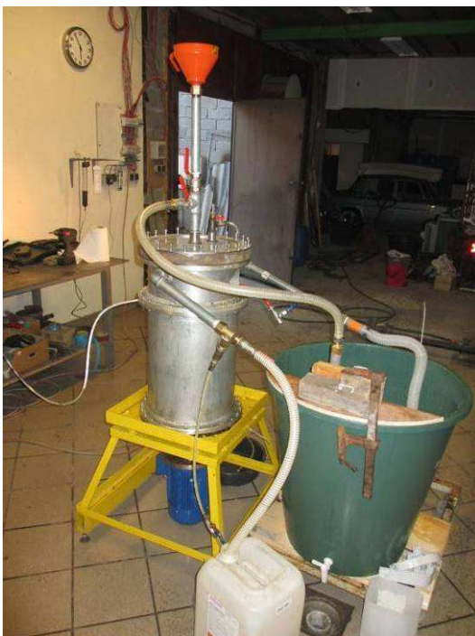
Figure 5: Experimental configuration for optimization tests in Ruffieux.
