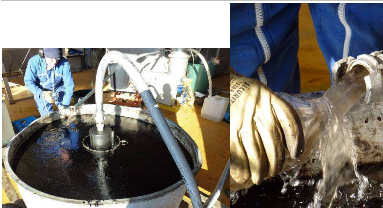
Figure 8: Water sampling at water outlet.
