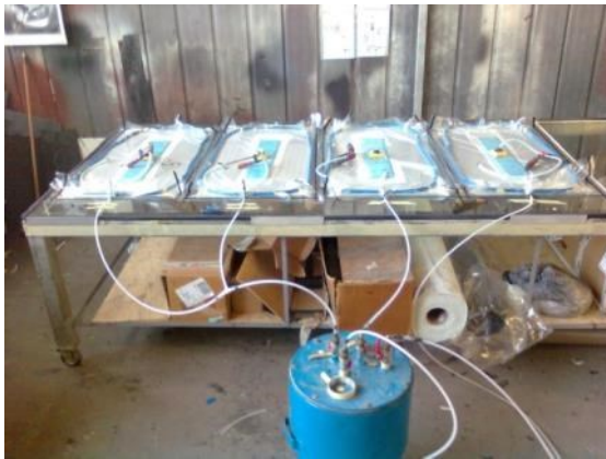
Manufacturing (left) and artificial aging (right) of P2 plate specimens
