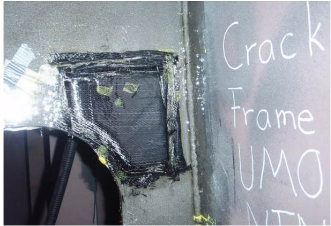
Vacuum infusion of patch repair inside the Catamaran (left) and finished patch (right)
