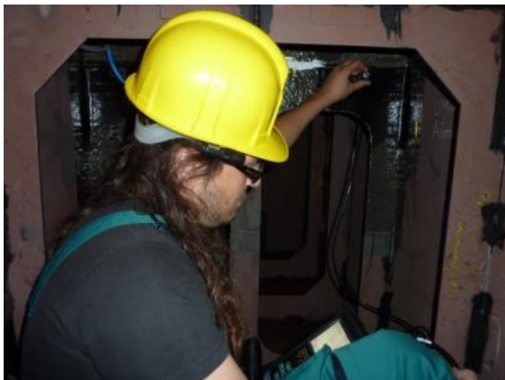
BondMaster acousto-ultrasonic NDE device applied to the Co-Patch full-scale catamaran application
