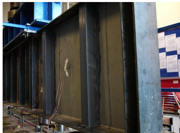
4-point bending test arrangement (left) and bonded composite beams against web breathing (right) in civil engineering applications steel girders
