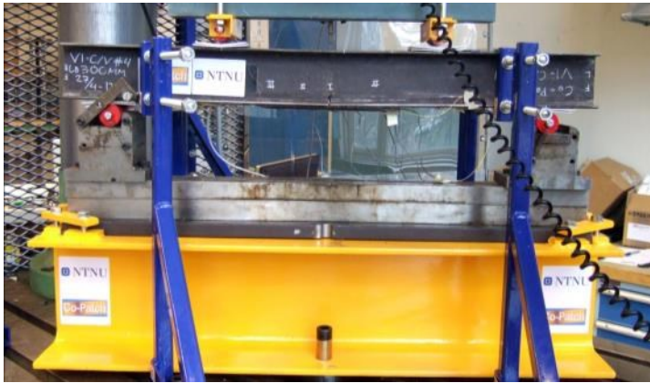
4-point bending test arrangement of patched beam specimens (left) and patch debonding (right)
