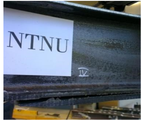
4-point bending test arrangement of patched beam specimens (left) and patch debonding (right)
