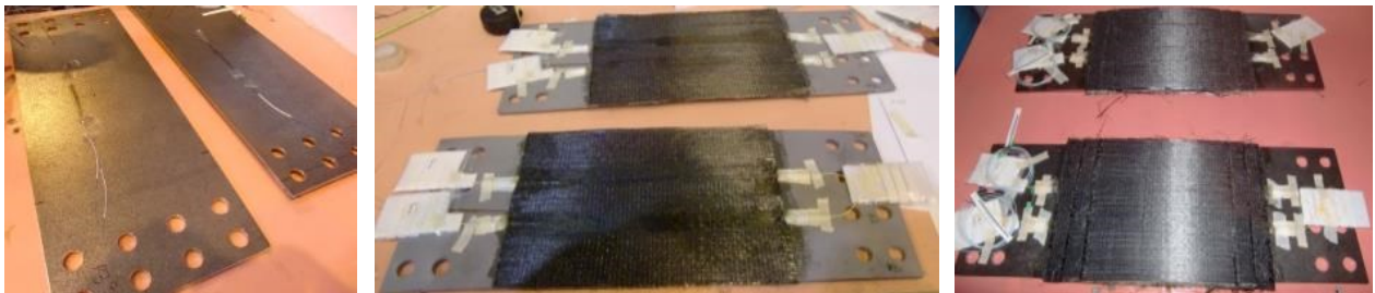
FBG attached to the steel (left), OBR applied to the CFRP composite patch (centre), embedded monitoring systems (right).
