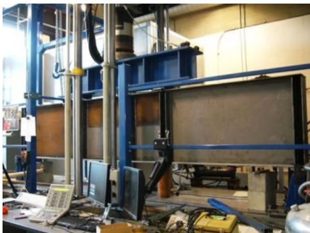
4-point bending test arrangement (left) and bonded composite beams against web breathing (right) in civil engineering applications steel girders
