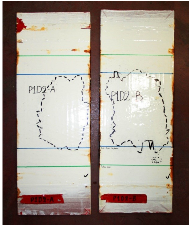
Findings in patched plate specimens after inspection with BONDMASTER device prior to testing
