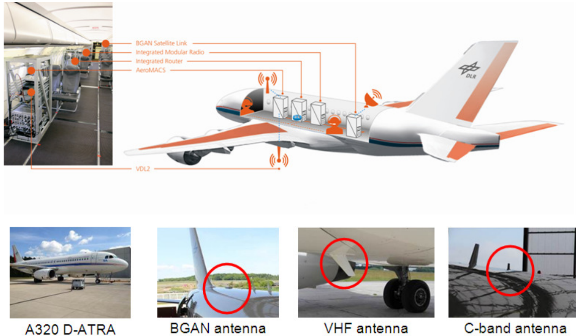
Figure 23: SANDRA airborne system installed in an A320 including the experimental antennas.
