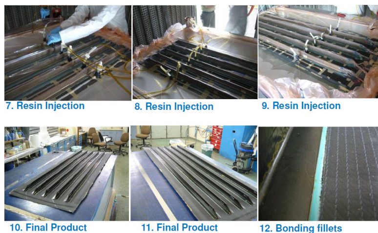
Figure 47: Wing box skin process flowchart part 2
