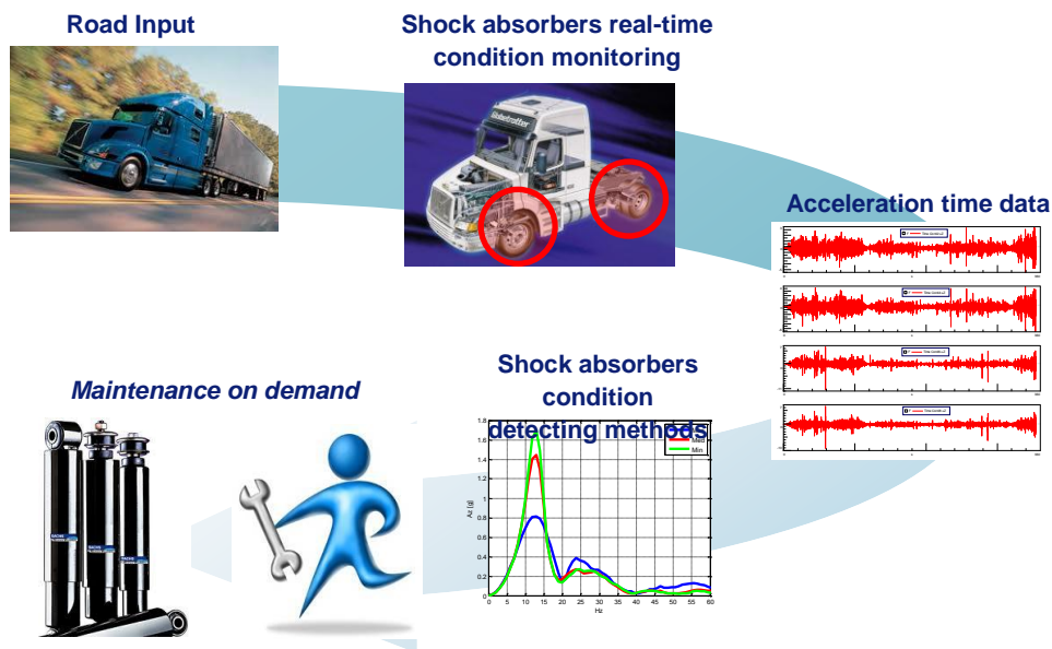
Figure 7: Shock absorber condition monitoring scheme.
