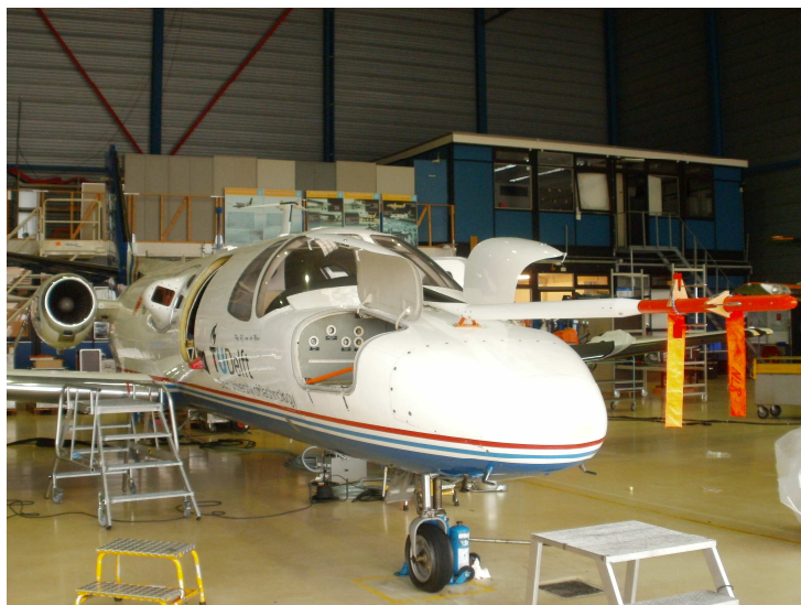
Figure 32 Test aircraft equipped with nose boom and fairing
