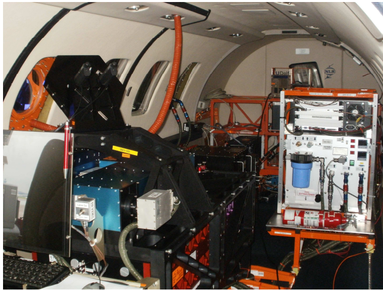
Figure 33 Lidar Installed on board the aircraft : left : Lidar rack – Right : Electronic rack
