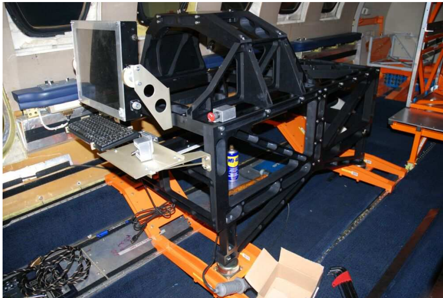
Figure 20 Lidar rack as integrated in the Citation 2 cabin in April 2012
