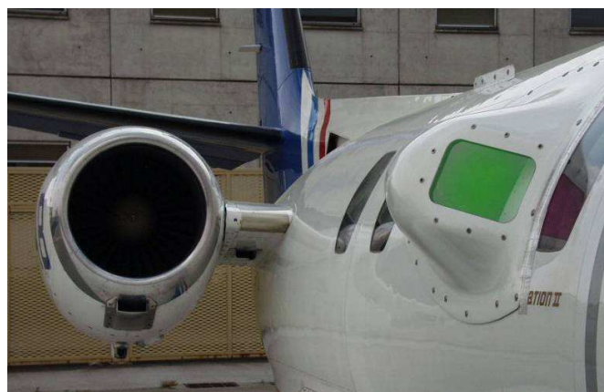
Figure 14 Fairing of NLR's Cessna Citation II
