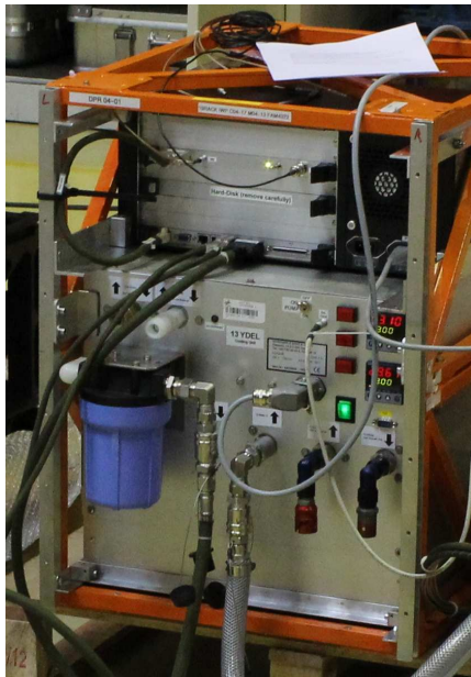
Figure 16 Left: Electronics rack containing the DLR data acquisition unit (top) and the heat exchanger unit (lower part) Right: Screen for lidar operator control attached to the lidar rack
