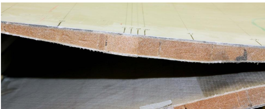
Figure 5: Different structures of composite materials used: a & c – “sandwich” structure; b – laminate structure
