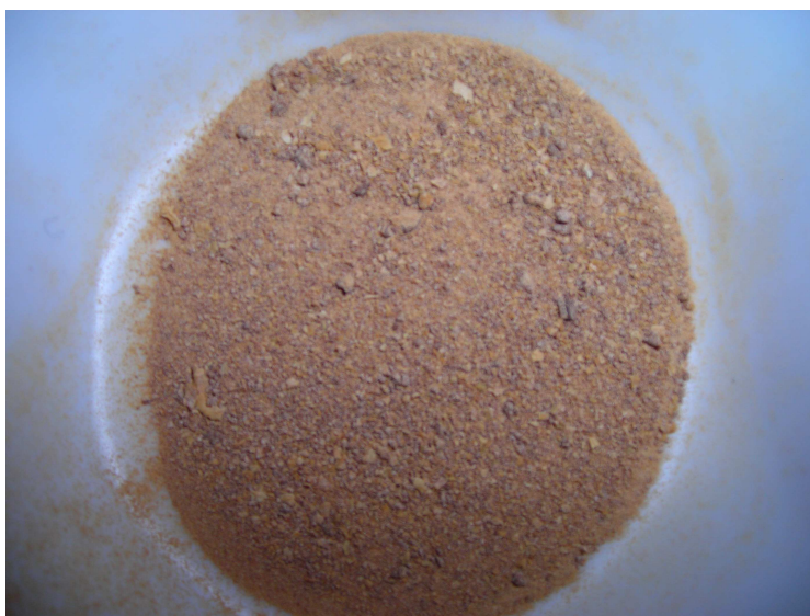
Fig. 13: Solid after the precipitation. It is red, because of iron precipitation
