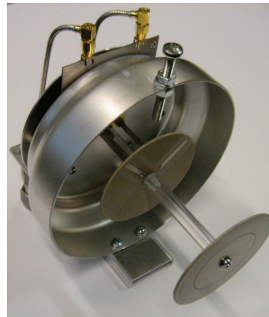
Parabolic dish feed with circular polarization and integrated low-noise amplifier.
