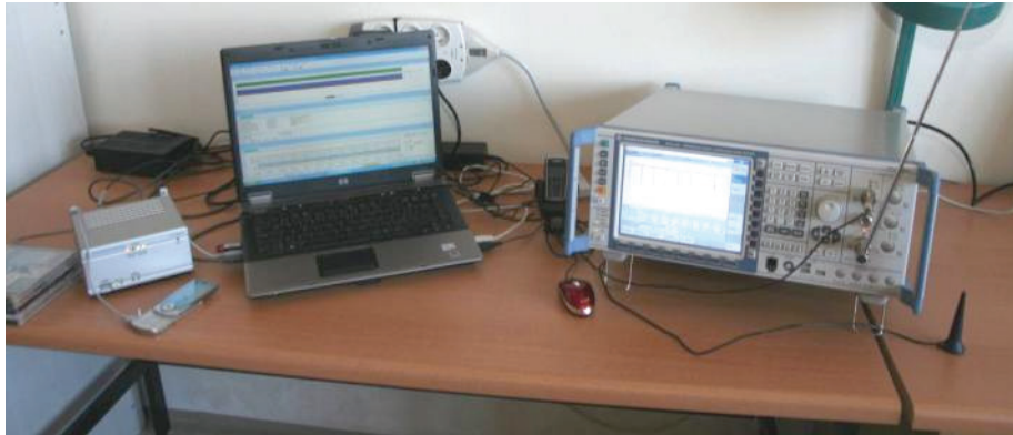
Throughput evaluation of the HSDPA transfer using the ROMES measurement system
