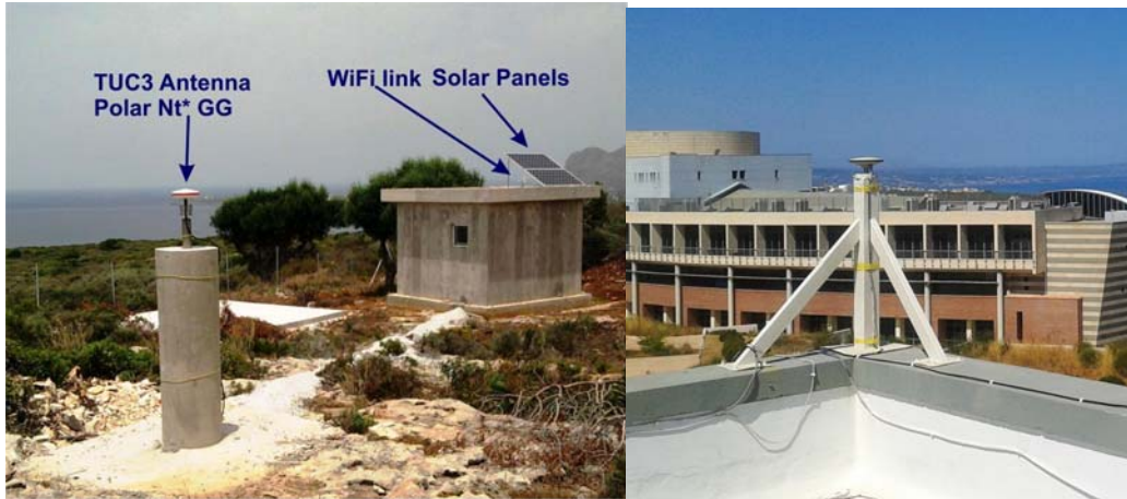
Figure 3. The “TUC3” Global Navigation Satellite System site of the European EGNOS (left) and the TUC4 BeiDou/Compass (right) chinese receiver sites at TUC facilities on campus.
