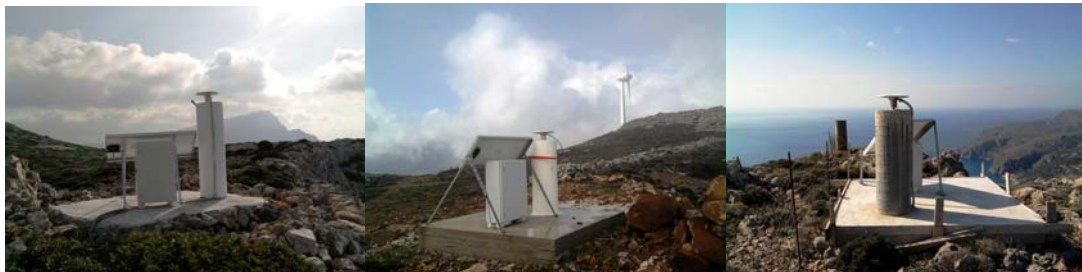
Figure 7. The “Menies” (MEN1), “Seli” (SEL1), and “Sougia”(SUG1)Global Navigation Satellite Systems permanent sites used for crustal deformation monitoring.
