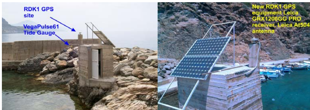
Figure 5. The instruments installed at “Rodakino” site, at a location along the ascending orbit of Jason satellite on the central west coast of Crete.
