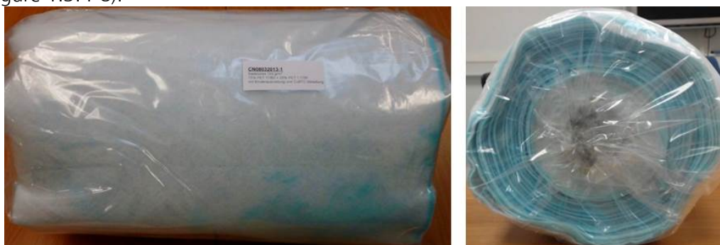
Figure 1.3.4-8: Continuously MOF-particle loaded PET-nonwovens for the demonstrator preparation (CuBTC <math><63 \mu\text{m}</math> from JM; loading capacity: 25 g/m 2 )
