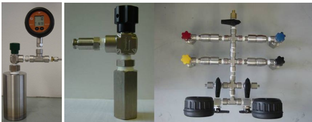
Figure 1.3.4-2: High pressure cylinder (200 ml) for storage and purification tests (left) and gas cylinder (15 ml) for high pressure tests (centre) and filling station (right).
