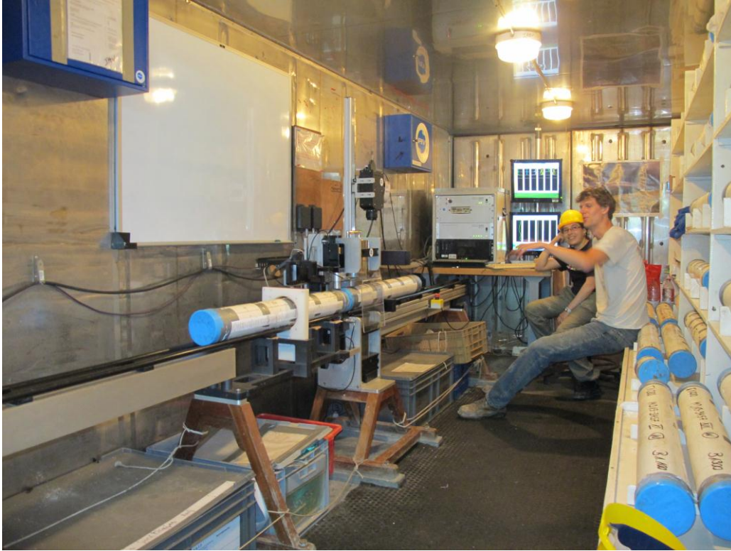
Multi-Sensor Core Logger (MSCL) room on board the French RV Marion Dufresne during the EUROFLEETS funded cruise TORE @ Laura Anton Lopez- IGME
