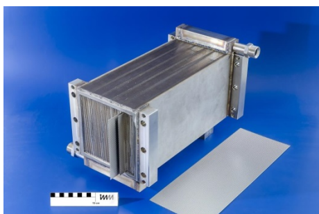
Fig. 29: Large laser welded stacked plate microreactor, comprising exchangeable roll embossed reaction plates of the size 150 x 400 mm. (Source: IMM)
