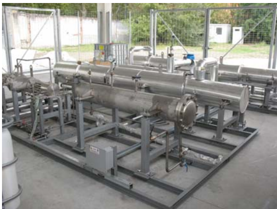
Fig. 18: Mini-plant for biodiesel production, located at Politecnico di Torino in Alessandria, Italy (Source: POLITO).
