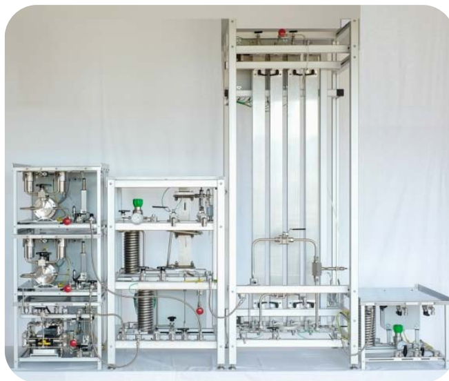
Fig. 13: Commercial Flow Miniplant for fast l/l reactions like epoxidation and propoxylation (Source: MIC).
