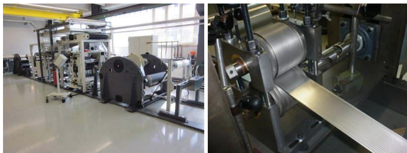
Fig. 25: Assembly for roll embossing at Wetzel company (left) and downstream side of the mating roll with a microstructured strip of 60 mm width (right) (Source: Wetzel GmbH).
