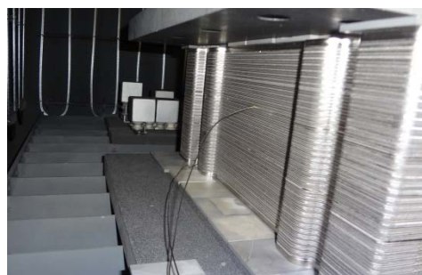
Fig. 30: Large stacked plate microreactor inside the vacuum furnace, comprising roll embossed reaction plates of the size (2x60) x 400 mm. (Source: IMM)
