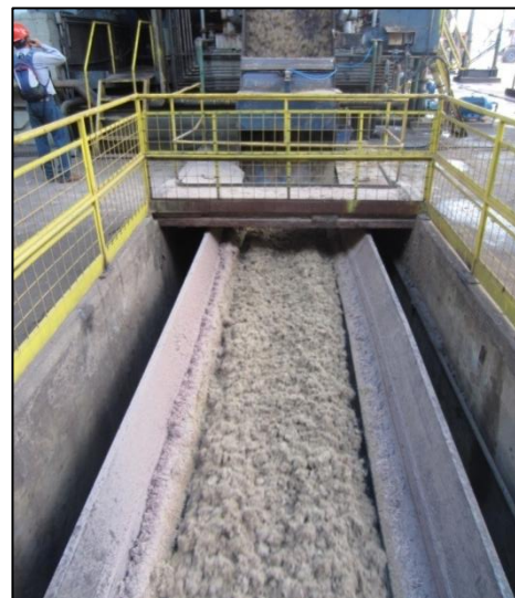
6. Bagasse which will be burnt for ethanol processing or electricity production
