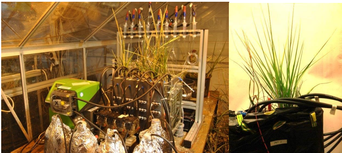
Stacked Plant-MFC in a greenhouse & plant-MFC with biocathode
