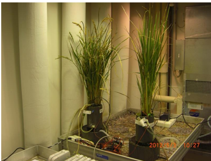
Photo of a tubular shaped Plant-MFC (anode in the central cylinder and cathode in the bottom cylinder) planted with rice and inoculated with the bacteria C. sporosphaeroides and G. sulfurreducens
