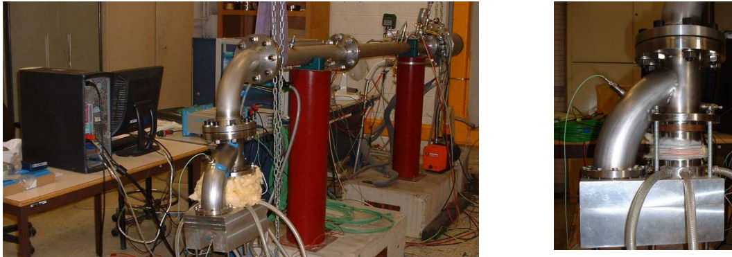
Figure 14 Overview of the refrigerator driven by the thermoacoustic prime mover
