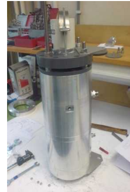
Figure 34 Set up used to determine the damping of the seal gap. The twin mass-spring systems will be tested separately
