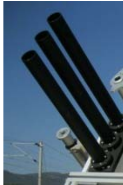
Fig. 12. Tri-band Spectro-heliometer sensors; Fraunhofer (left) IES-UPM (right)
