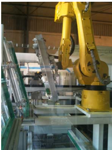
Fig. 21. Robotic arm for SoG lens parquet placing
