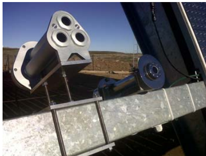
Fig. 13. IES-UPM Tri-band Spectro-heliometer in Morocco (left) and Egypt (right)
