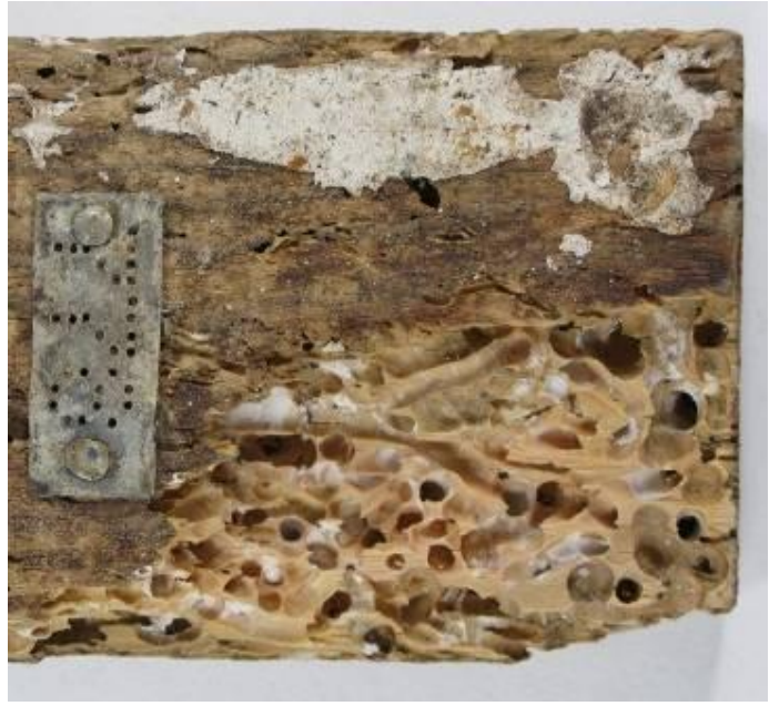
Figure 2. Heavy attack by Teredo navalis . The mollusc penetrates and digests the wood material forming up to one centimetre wide tunnels.
