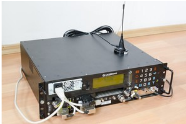
Figure 21 - Independent Digital Repeater (IDR) from Cassidian
