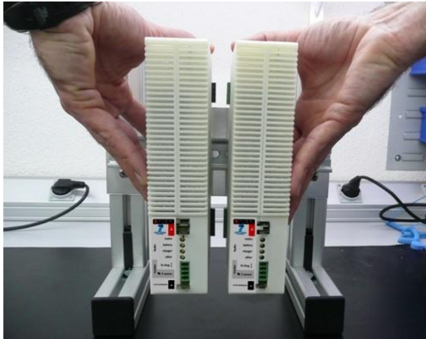
Showing how the modules are “stacked”, by pressing them together, with 5.08mm Eurostyle connectors at the rear proving electrical connection and mechanical support
