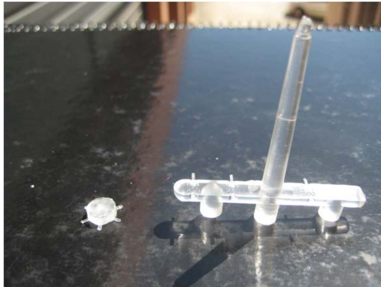
Fig. 7: Comparison between the samples made by conventional injection (right) and ultrasound injection (left)
