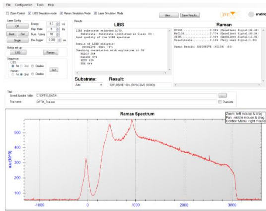
Figure 27. Screenshot of the final version of the User Interface of the OPTIX prototype.
