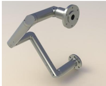
Figure 21. Articulated Optical arm for the OPTIX prototype.
