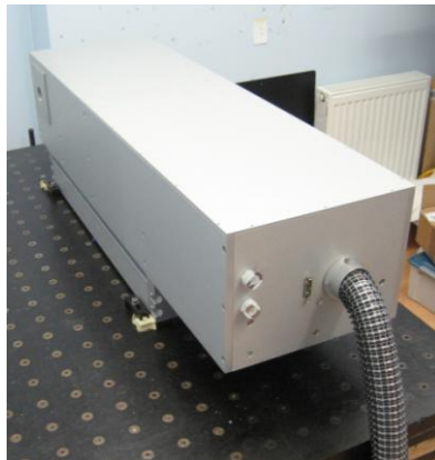
Figure 16. NL310 laser rear view. Connectors for cooling tubes, power cable umbilical and control socket are visible
