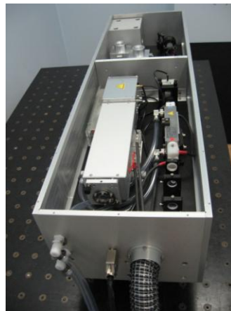
Figure 18. NL310 laser view with upper covers opened.
