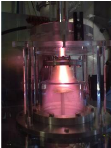
Fig 26 Plasma source implemented at University of Padua-CISAS to study surface modification due to plasma surface interaction using S-Helicon antenna.
