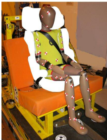
UNECE Reg.44 testing bench
