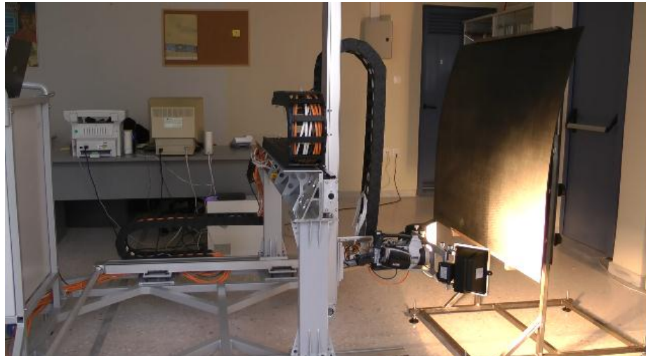
Figure 21. ComPair Inspection procedure of the CFRP sample
