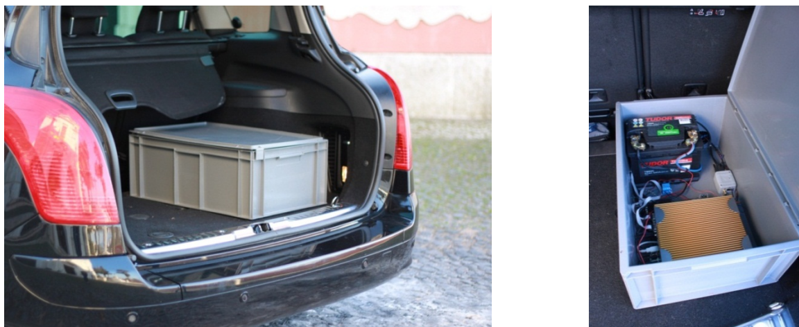
Figure 6. The secure housing of the PC onto which all data was recorded; mounted in the boot of each of the instrumented vehicles.
