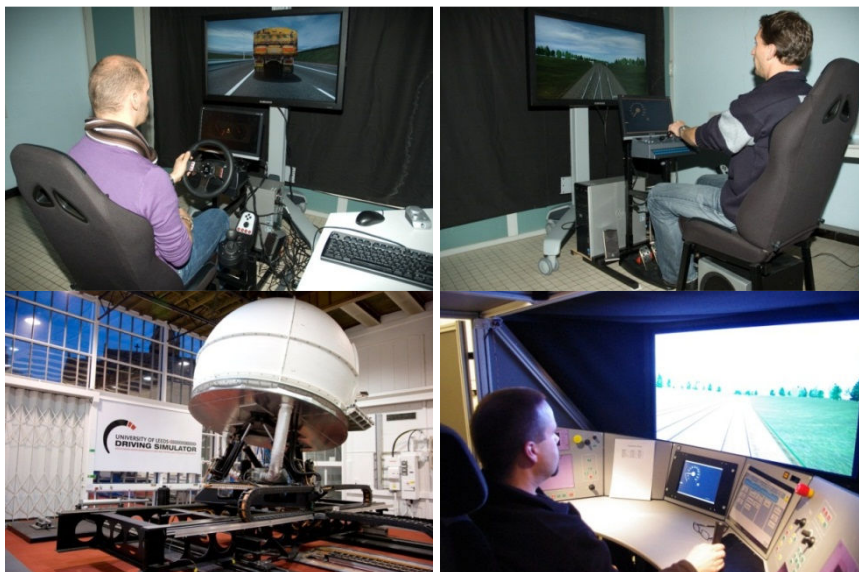
Figure 2 Simulators used (top left - small scale car simulator, top right - small scale train simulator, bottom left – full scale car simulator, bottom right . full scale train simulator)
