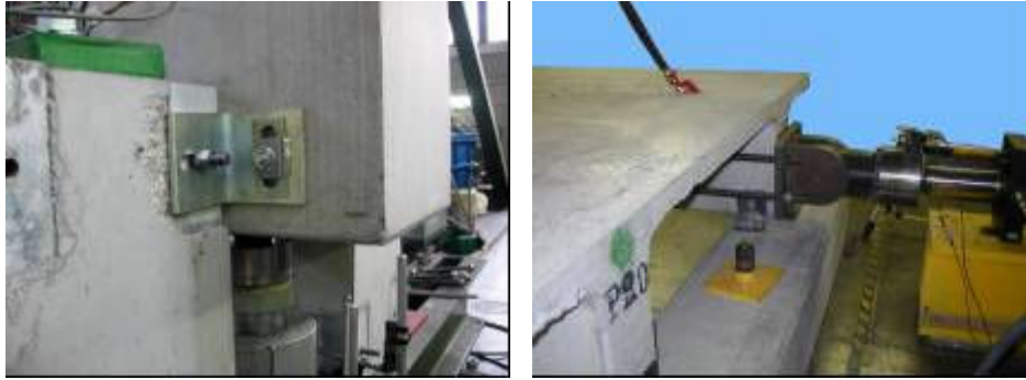
Figure 1 - Floor-to-beam connections: local tests and tests on subassemblies
